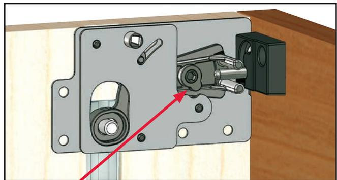
Lock arm adjusts vertically +/- 3/16" for ease of alignment. Lock arm adjusts with 5/32" hex wrench. Low profile actuator fits within 1/2" drawer suspension.
