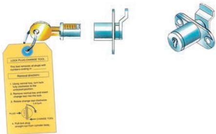
A change tool (P/N KY-500) is required to remove plugs. A firm clockwise turn removes the plug.
