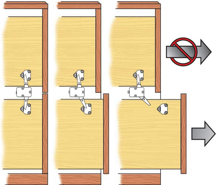
WHEN EITHER DRAWER IS PULLED OPEN, THE DRAWER CLIP ON THAT DRAWER MOVES THE SNAPPER INTO A LOCKED POSITION... THEREBY PREVENTING ANY FURTHER DRAWERS FROM BEING OPENED
