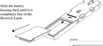
Install four AAA batteries in the slots indicated on the back of the battery housing.
