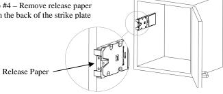
Step #5 – Close door firmly and open it again. The strike plate will become affixed to the door in the proper mounting position. Remove and discard red installation tool
