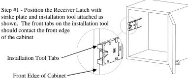
Step #2 - Screw the Receiver Latch in place using 2 of the #6 x  $\frac{1}{2}$ " screws supplied, in the front side of the oval holes. If attaching to material less than 34" thick, alternate fasteners may be required.
