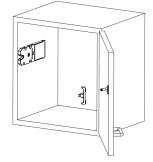
Step #6 - Screw the strike plate in place using 2 of the #6 x ½" screws supplied. If attaching to material less than 3/4" thick, alternate fasteners may be required.
